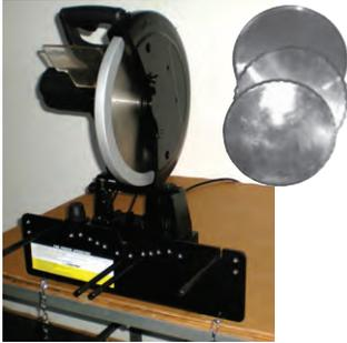
This cutting machine easily handles all 1 and 2 braided wire hose through 4" I.D., up to 2" I.D. 4-spiral and up to 1-1/2" I.D. 6 multi-spiral reinforced hose. That makes this machine ideal for cutting most hydraulic and pneumatic hoses as well as a variety of industrial fluid transfer hoses. The T-71 uses a 14" cutting blade, T-1070, for cutting all 1 & 2 wire braid and through 2" 4 spiral hose. The scalloped toothed blade T-1071, is for cutting industrial
