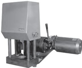
The T-400-PH conversion kit is designed to allow the use of standard Weatherhead Coll-O-Crimp tooling, hose, and hose ends in the Parker 80c crimper. Everything is included to convert the crimper to accept Weatherhead tooling. This kit gives the crimper capacity to crimp up to and including 1-1/4" I.D. 2-wire hose factory-type hose assemblies.
