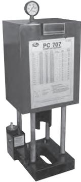
The T-400-GT conversion kit is designed to allow the use of standard Weatherhead Coll-O-Crimp tooling, hose, and hose ends in the Gates PC707 crimper. Everything is included to convert the crimper to accept Weatherhead tooling. This kit gives the crimper capacity to crimp up to and including -10 I.D. 2-wire hose factory-type hose assemblies. **This kit does not include the T-400-8 die ring which is required for crimping.**
