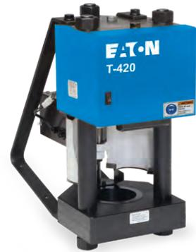
The T-420 is a versatile machine ideal for your shop, factory, construction, and mine locations. Large capacity combined with lever-activated crimping gives you wide coverage and a quick and simple way to make factory-quality hose assemblies.
